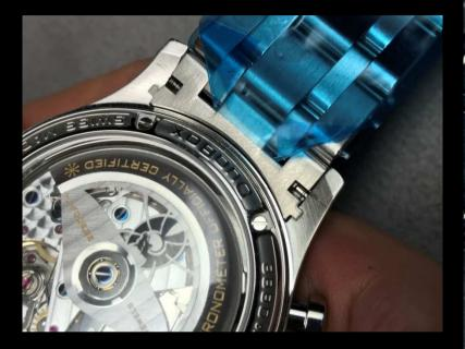
5. Once the two bars are in position, press the end piece slightly while holding it close to the case, until it clicks, which means that the spring bar is in position
