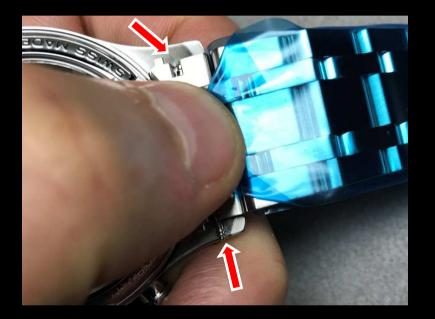
4. Using the mounting tool, while holding the bracelet in its position, gently press the head of the spring bars to place them in to horns, one side after the other
